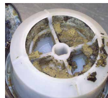
Centrifuge drum, performance hampered by sludge
