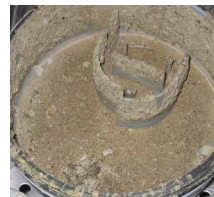
Separation tank, full of sludge
