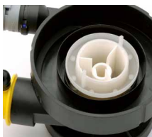
Centrifuge housing, encrustation is ruled out here
