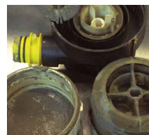
Centrifuge housing, encrusted - total breakdown of the suction unit
